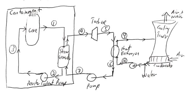
Fill out the table detailing the various streams in the simplified PWR reactor. Calculate the overall efficiency for the plant (Net  $W_s/Q_{Core}$ ) Ignore the shaft work for the cooling tower cycle. Use linear interpolation to find the values from the steam tables. Compare the efficiency of this PWR with that of a Carnot engine. (Note: GW = 1e6 kJ/s).
